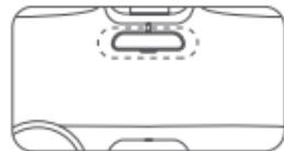
Avoid the edge of the windshield and select the flat and smooth area for the installation.
