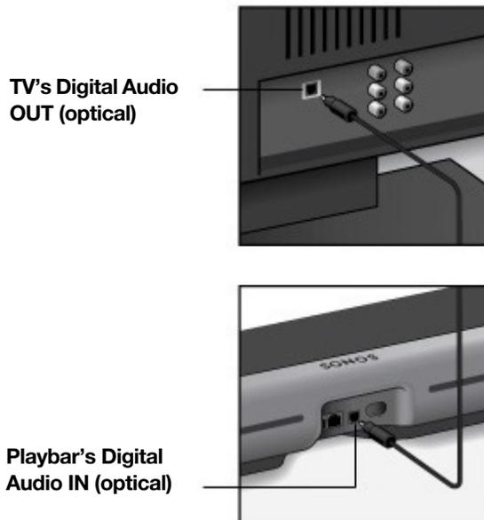
**IMPORTANT:** Remove the protective caps from each end of the optical audio cable before inserting.
