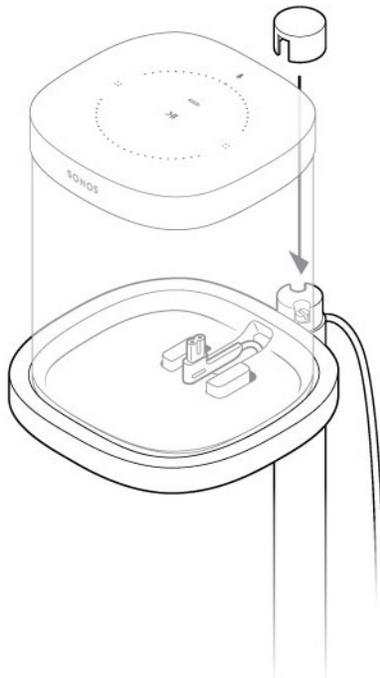
6. Press the power cord into the stem, working from top to bottom. Pull the excess cable down from the base.
