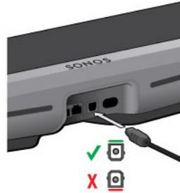
Optical input supports Dolby Digital and stereo.
