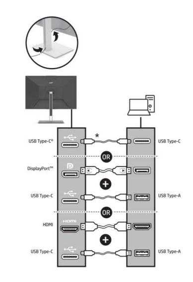
**NOTE**: Both camera and microphone function only if the monitor is connected to the computer as shown in the illustration.
