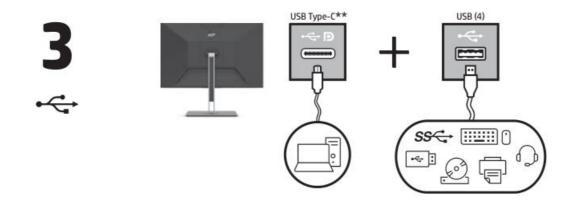
\*\*The USB hub is enabled only if the monitor is connected to the computer via the USB Type-C to Type-C cable (included) or a USB Type-C to USB Type-A cable (sold separately).
