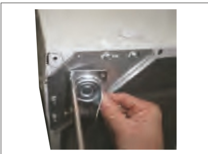
5、 Fix the casters by screwdriver.
