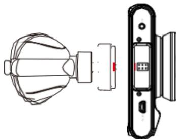
Holder base the other side have only 1 gap also must be fit into camera body 1 clip
