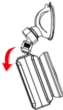
Please remove the camera body clips from the holder base gap like the graphical direction
