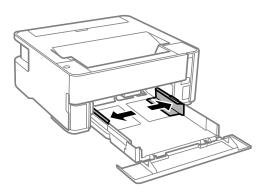
4. With the printable side facing down, load paper until it touches the back of the paper cassette.
