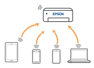
The printer can be connected by Wi-Fi or Ethernet, and Wi-Fi Direct (Simple AP) connection simultaneously. However, if you start a network connection in Wi-Fi Direct (Simple AP) connection when the printer is connected by Wi-Fi, the Wi-Fi is temporarily disconnected.
