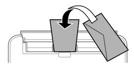
Load envelopes in the paper cassette with the flap facing up, and then slide the edge guides to the edges of the envelopes.
