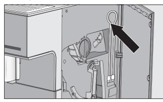
The milk tube for cartons and other suitable containers is located behind the appliance door.
