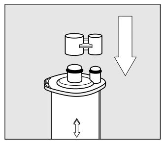
■ Seal the cartridge with the cap.
