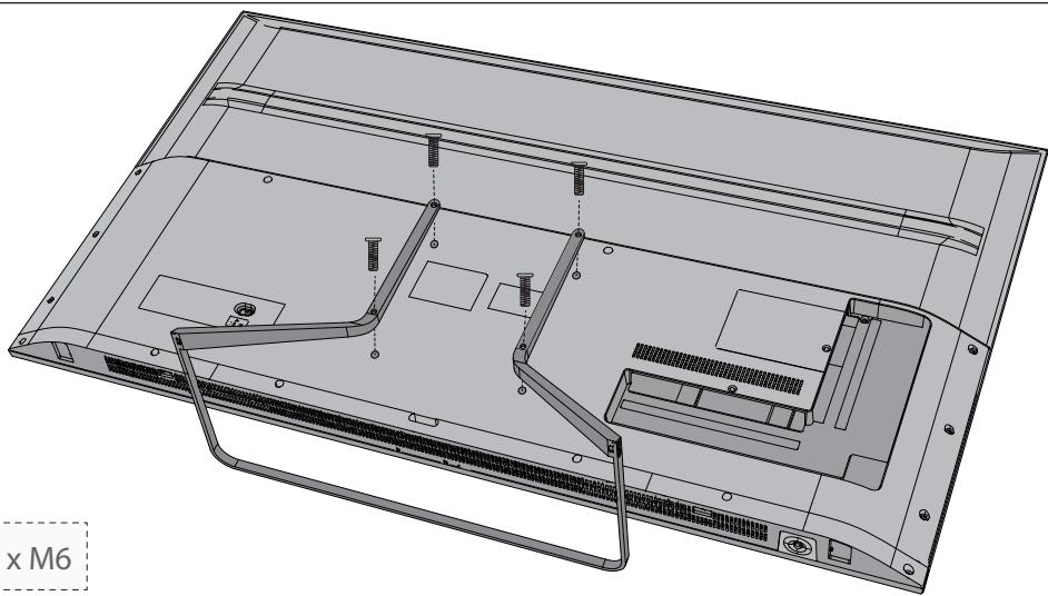
**English:** To assemble the base stand to the TV you will need a cross head screwdriver. To avoid damage to the TV screen during assembly ensure the TV is placed on a soft flat surface with the LCD screen facing downwards.
