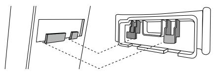
2. Slide the cable holder to the right, and attach it to the stand.
