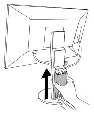
2. While holding down is of (A) lightly, slide (A) upward to detach it from the stand.
